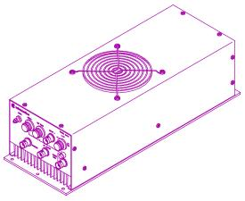
output envelope, is provided. The fault/interlock circuit which can be connected to the thermostat of a Q-switch will latch the power supply off when an open condition is present. High VSWR, over power, and low power indicator options are available.
